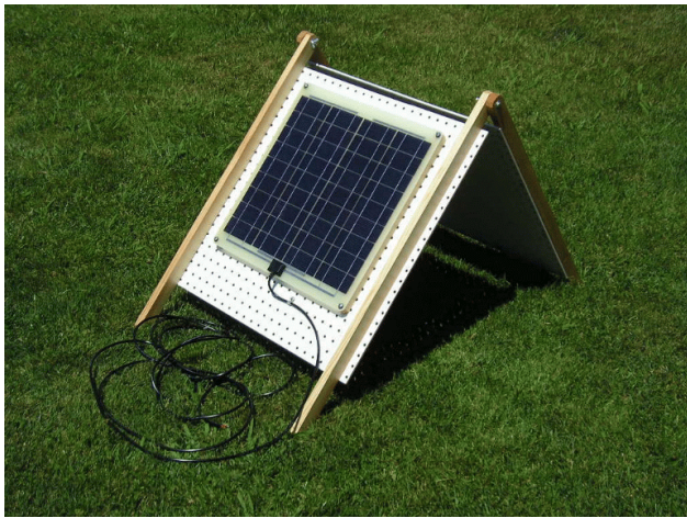
Photo 4. When the legs are folded back about 270 degrees, the panel is oriented for maximum sun exposure.
